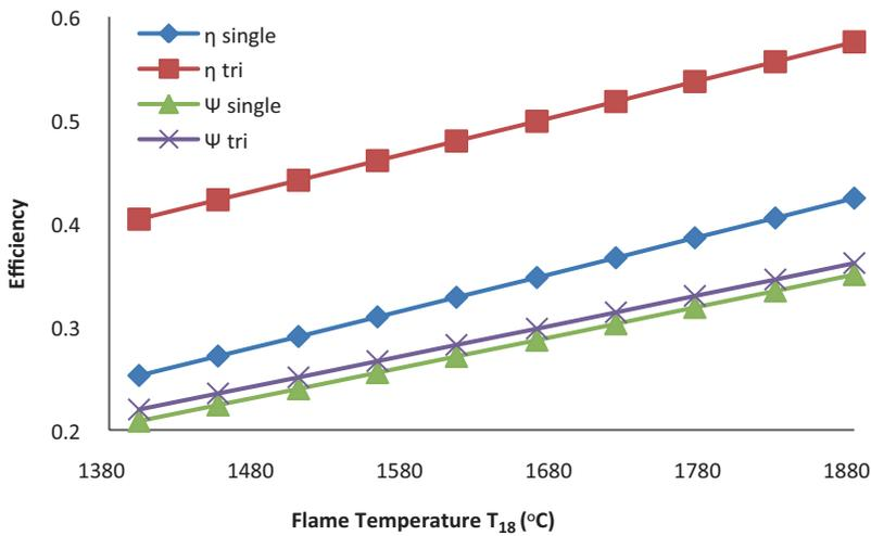
Fig. 5.12 Effect of CC outlet temperature on efficiencies
